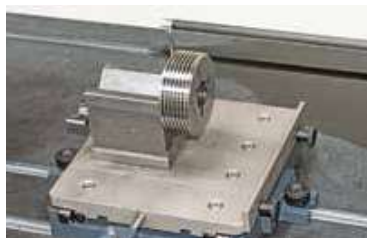
Thread Form checking on Zeiss Surfcom Contour Measuring instrument.
