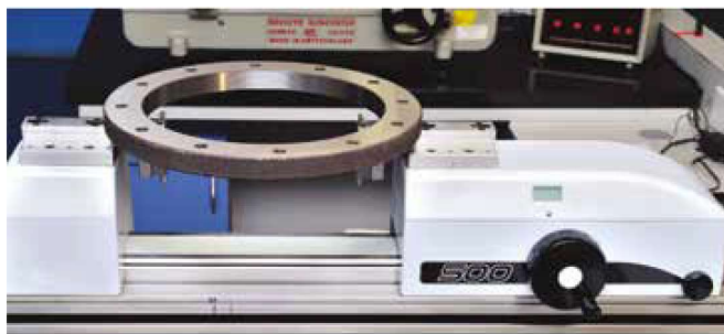
Thread Ring checking on SIP Universal Length measuring instrument.
