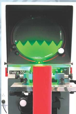
Measurement of Angle on Profile Projector
