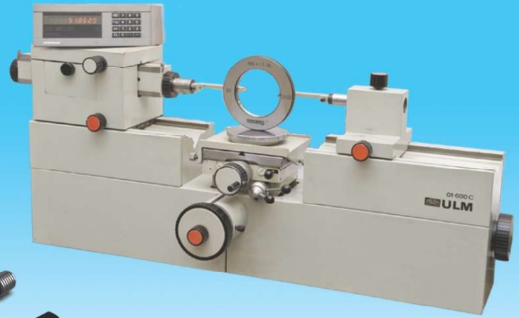
Measurement of Thread Ring, Gauge
