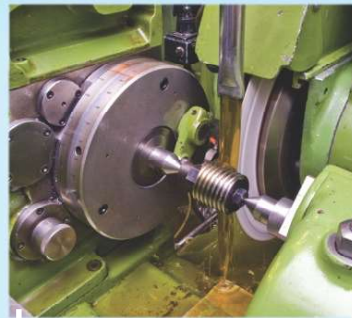
Thread Grinding of Plug Gauge
